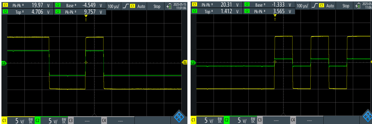
Figure 82 Test 2 of -4.5V which still passed (left), and tests 4 and 5 of 1.33V which failed (right)
