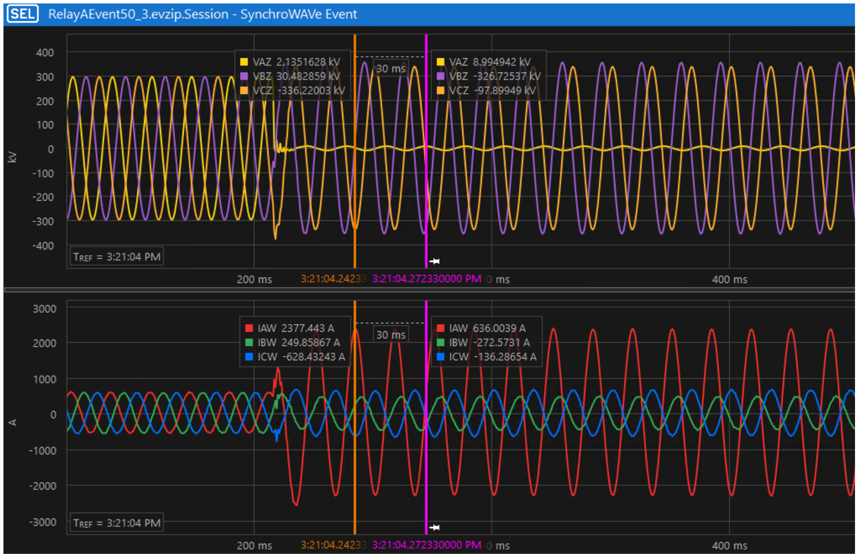
Figure 154. Fault calibration testing of SCALING values – Relay B – Bus 39
