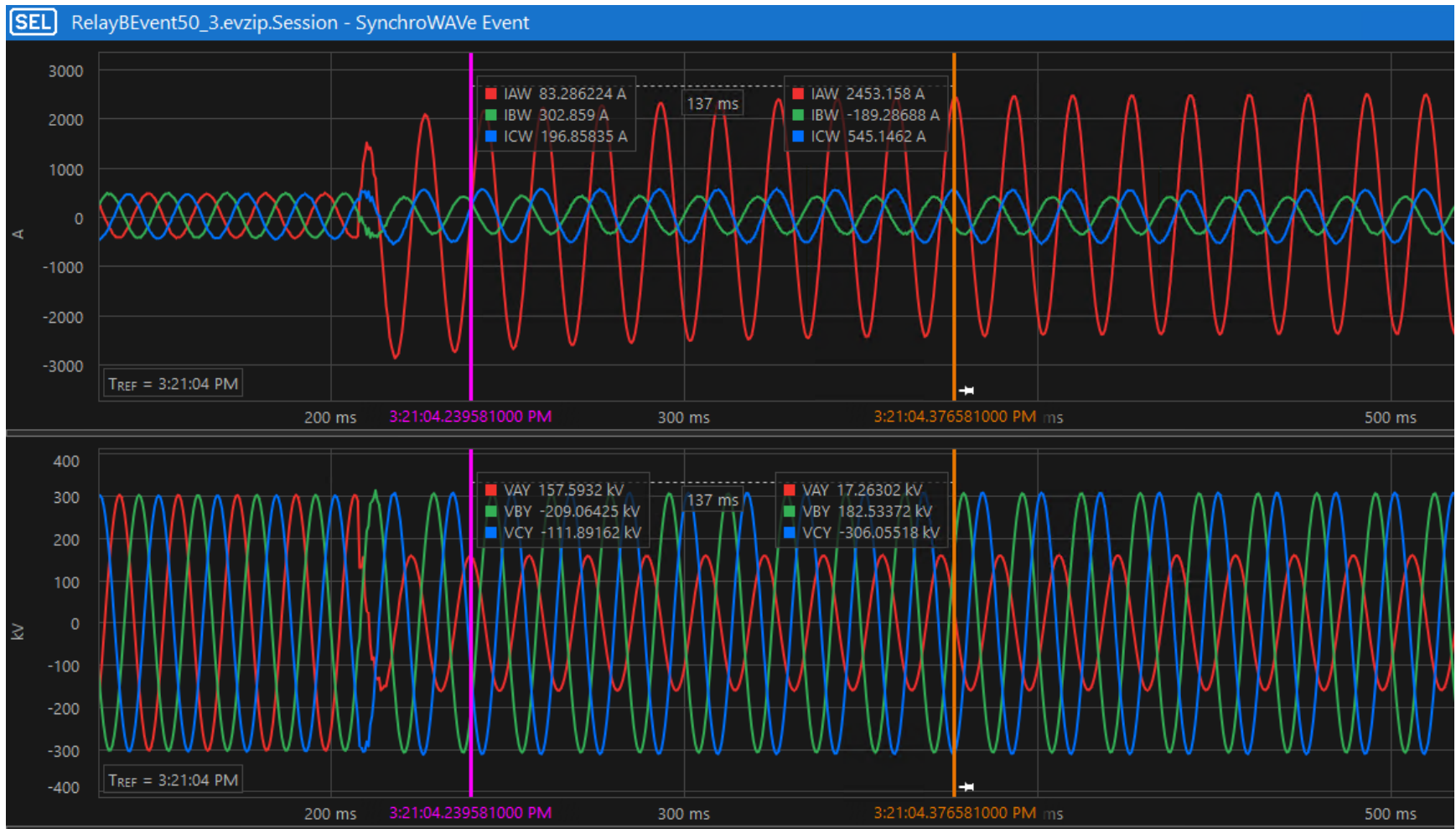
Figure 155. Relay B event file for SLG fault for calibration
