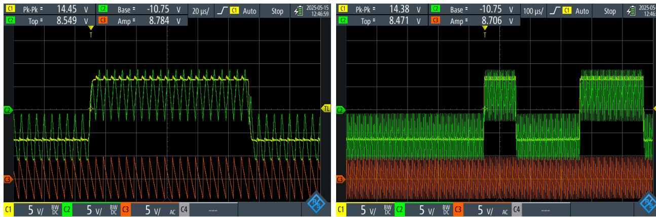
Figure 87. Sawtooth noise patterns that caused signals to fail. Sawtooth pattern with large period (left), and pattern with smaller period (right)
